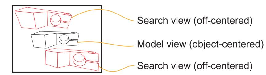
Refine the pose by minimizing the distances between the image edge points and the projected model edges
