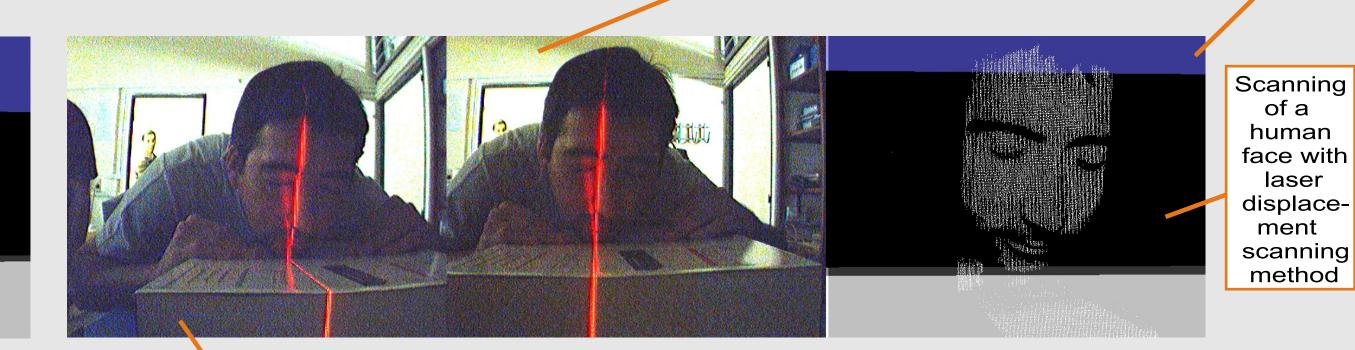
Laser scan data acquisition: In this case, the object to be reconstructed remains fixed, while its surface is revealed by scanning the area with a laser. It is intended for objects with no volume of revolution or whose content is shown by a single face.
