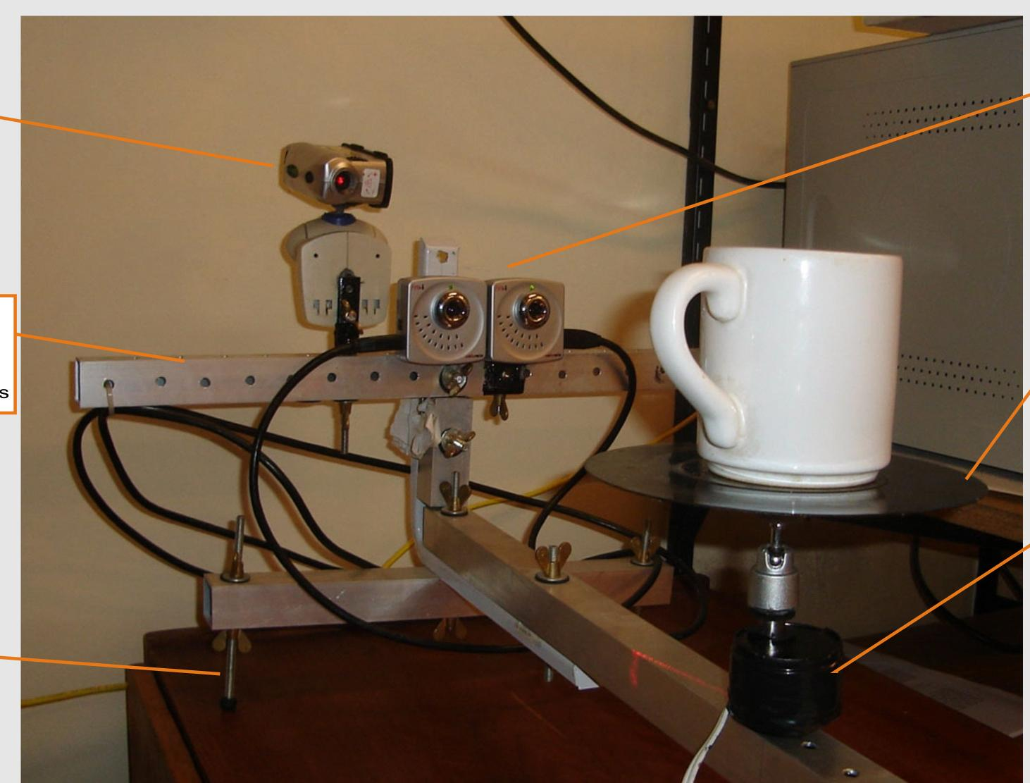
The stereo capture is made with two 30 fps, 640x480 webcams. It is necessary to calibrate the cameras intrinsically and extrinsically only once
