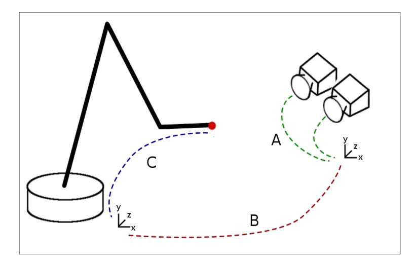
This map is invertible. The robot can place its hand anywhere in the scene it can find a point match, and also locate its hand in each camera.
