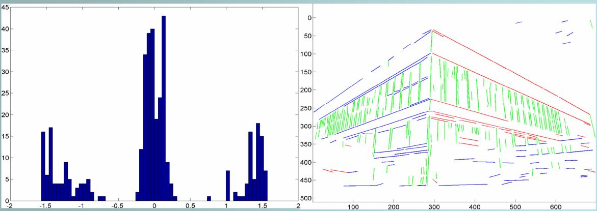
After fitting a curve to the orientation histogram of the line segments, three highest and well separated peaks were selected. Line segments with orientation in the range of [-pi/8 pi/8] around each peak were grouped together. Initial vanishing points location within each group were calculated using:
