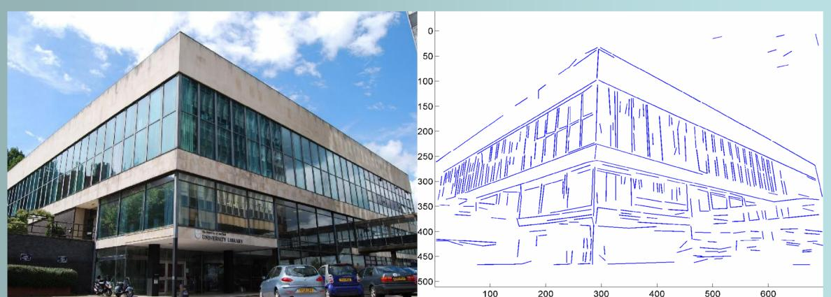
Under projective transformation, the parallel lines of buildings intersect at vanishing points in the image. The line segments were detected, short segments were eliminated since they are more likely to be clutters.
