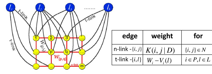
Minimizing E(f|D) is equivalent to finding a minimum cost multi-way cut in the graph shown above.
