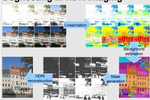
We adapt our method in order to handle image sequences with varying exposure time. First, we linearize the input images, and then estimate the background in the irradiance domain. We use the estimation to generate background masks and compute a deghosted[4] high dynamic range image.
