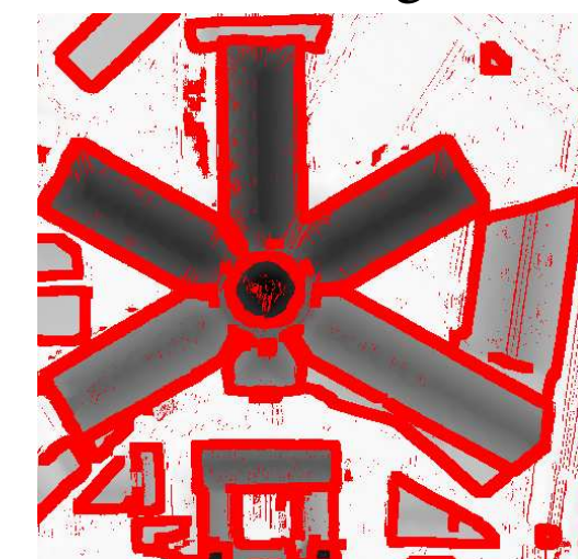
Disparity. Red pixels aren't matched (rejected by the a contrario method or the fattening correction.)
