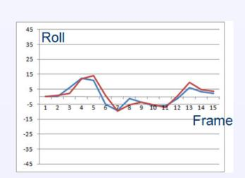
Result of testing. Blue lines - estimated angles, red lines - real angles.
