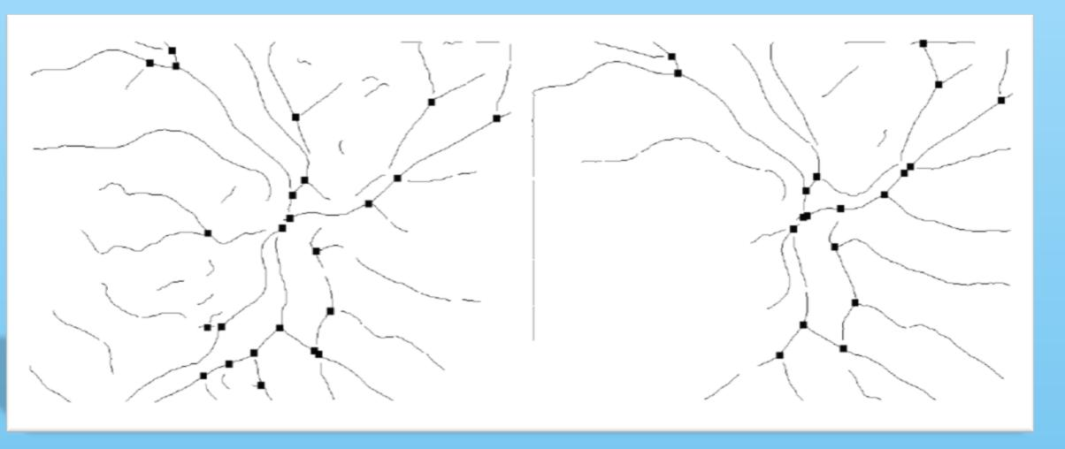
Once the patters are aligned, two points of different patter match if the distance between them is smaller than a given threshold, Dmax. Using the number of matched points a similarity metric, Sy, can be established.
