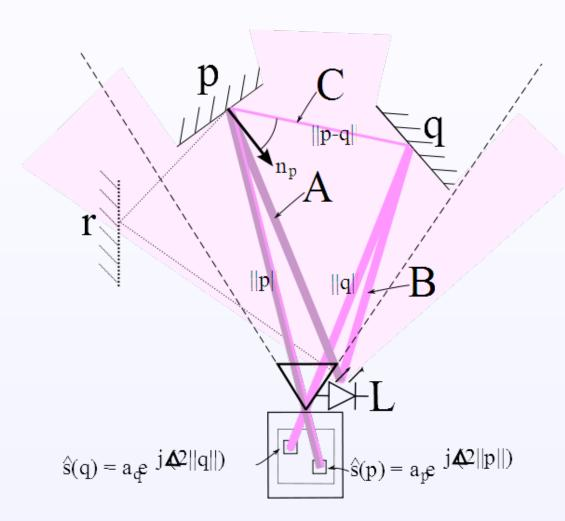
The diagram illustrates a luster cone not being congruent with the camera's field of view (dashed line). In this case, the unseen surface **r** also influences the measurement (dotted line).
