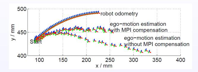
The measured and estimated trajectories are plotted in the diagram. The ego-motion-estimation without MPI compensation shows a large deviation. Applying the MPI compensation reduces the localization error from 140 mm to 60 mm and from  $2.5 ^{\circ}$  to  $0.5 ^{\circ}$ .
