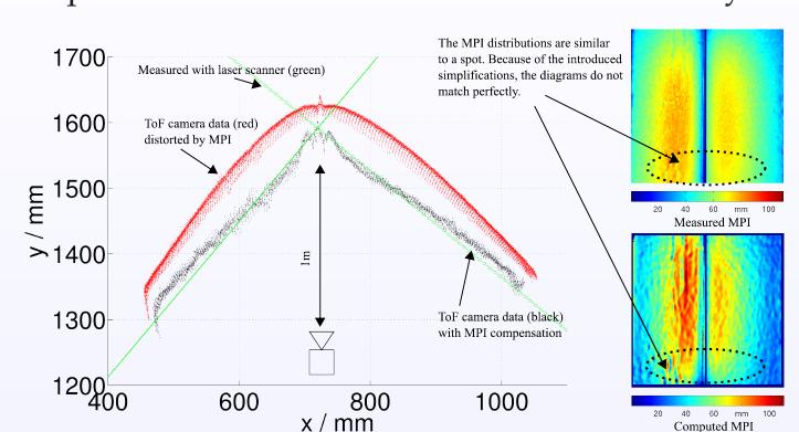
Applying the MPI compensation reduces the root mean squared error from 57 mm to 17 mm (black). The right diagrams illustrate the measured (top) and computed MPI related error (bottom) in this corner scene.
