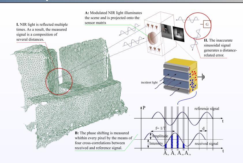
Schematic illustration of the measurement principle and its basic error sources. The distance-related error arises inside the camera, whereas the MPI is defined by the scene configuration.
