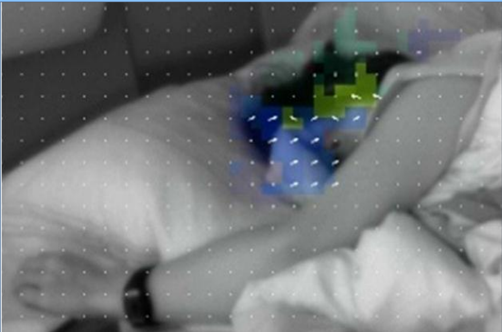
Figure 2. Resulting color-coded motion vectors from the processed video images. Blue area: hand moves to the right. Green area: head moves to the left.
