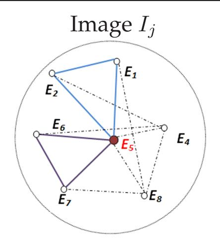
The two plain triangles  $(E_1, E_2, E_5)$  and  $(E_5, E_6, E_7)$  satisfy the  $\Delta$ -TSR constraints. Note that  $E_4$  significantly moves in  $I_i$  and  $I_j$  while all other points slightly move and that  $E_3$  disappeared and  $E_8$  appeared in image  $I_j$ .
