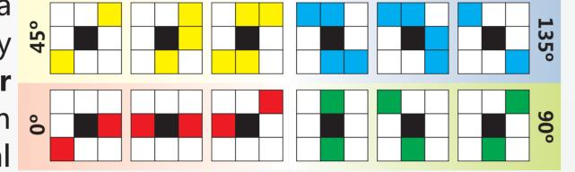
geometrical structures similarly to grayscale Local Binary Patterns [2]. Every active (contour) pixel encodes a N-bit LCP word (N=3 in our example) encoding neighborhood information. For Traffic Sign Detection only some code words representing linear structures with selected angles are meaningful, so they can be grouped in 4 sets of directions, which we call Condensing Codes (CC).
