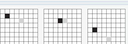
level comparisons between pixels of the image at training resolutions. All possible pixel combinations are taken into account, and opposed to Haar features, involved zones do not have to be adjacent. Original Haar-Like features (or more complex Dissociated Dipoles [5, 6]) can be decomposed into a finite combination of Quantum features. Their versatility makes them extremely flexible for multipurpose detection tasks.
