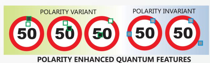
This representation allows more compact and efficient detectors, and can be effectively meaningful for Traffic Sign Detection.
