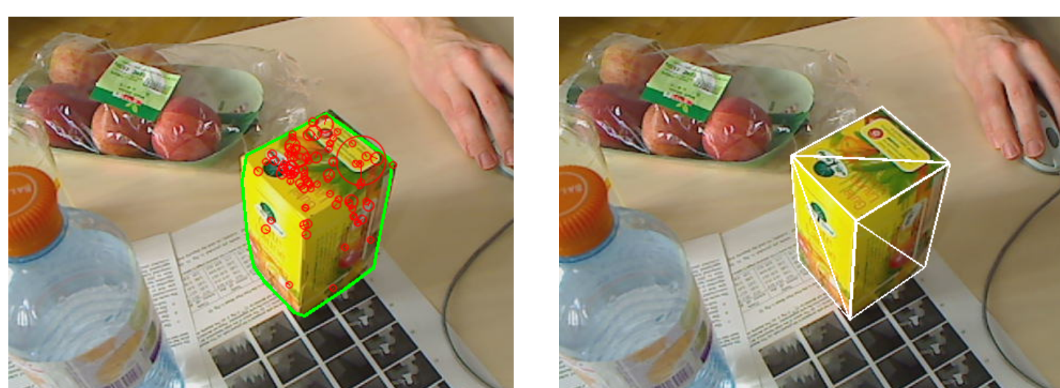
Figure 4: Recognition of SIFT and pose estimation (left) and reinitialised tracker (right)
