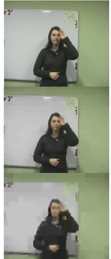
Fig. 4. Picture taken from experiment: first is original next decoded frames by H264 codec with parameter QP40, 50.
