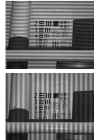
**Problem** The difference in viewpoint between the camera and projector, induces scene-dependent lateral displacements and frequency changes in the periodic pattern. This forms the basis for *depth estima*tion using Structured Light [3].
