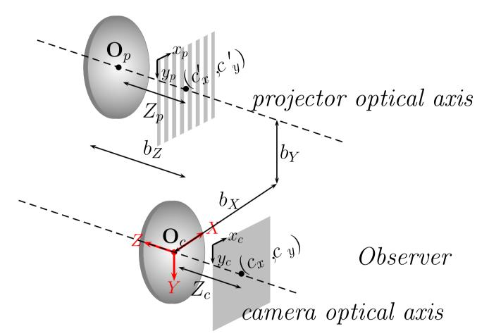
Illumination  $s_{\theta}(x',y') = \frac{A}{2} + \frac{A}{2} sin \left(2\pi \left(\frac{\xi_0}{N_p}x' + \frac{\eta_0}{M_p}y'\right) + \theta\right) \begin{vmatrix} M_p, N_p & \#rows, columns in projected image \\ (\xi_0, \eta_0) & spatial frequency of pattern \end{vmatrix}$ camera image of size  $N_c \times M_c$
