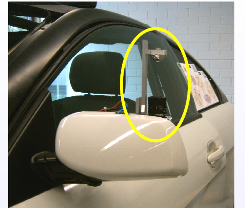
Omnidirectional camera integrated with the side-view mirror of the car
