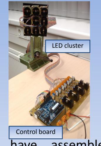
We have assembled a system comprising multiple LEDs with different spectra to illuminate a scene using a conventional RGB camera to acquire the images.
