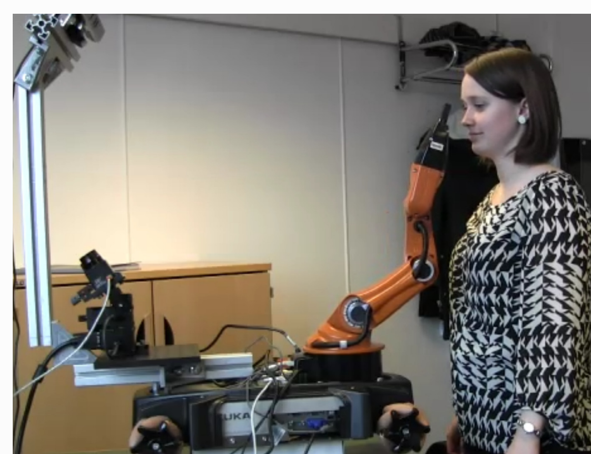
Experimental setup with KUKA youBot, Microsoft Kinect 3D sensor and human obstacle.
