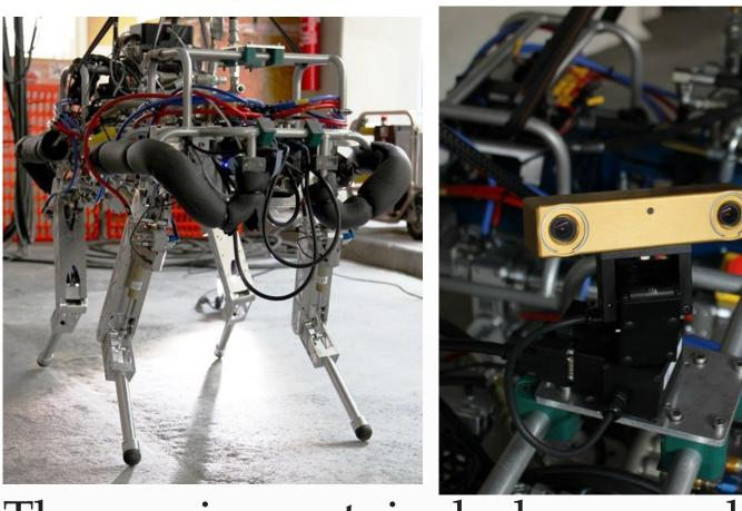
The equipment include as on-board vision system a Pointgrey Bumblebee Camera and a FLIR D46-17 PTU
