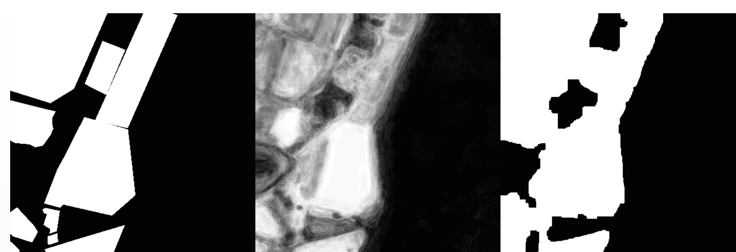
From left to right: hand labels, RF class probabilities, and graph cut segmentation
