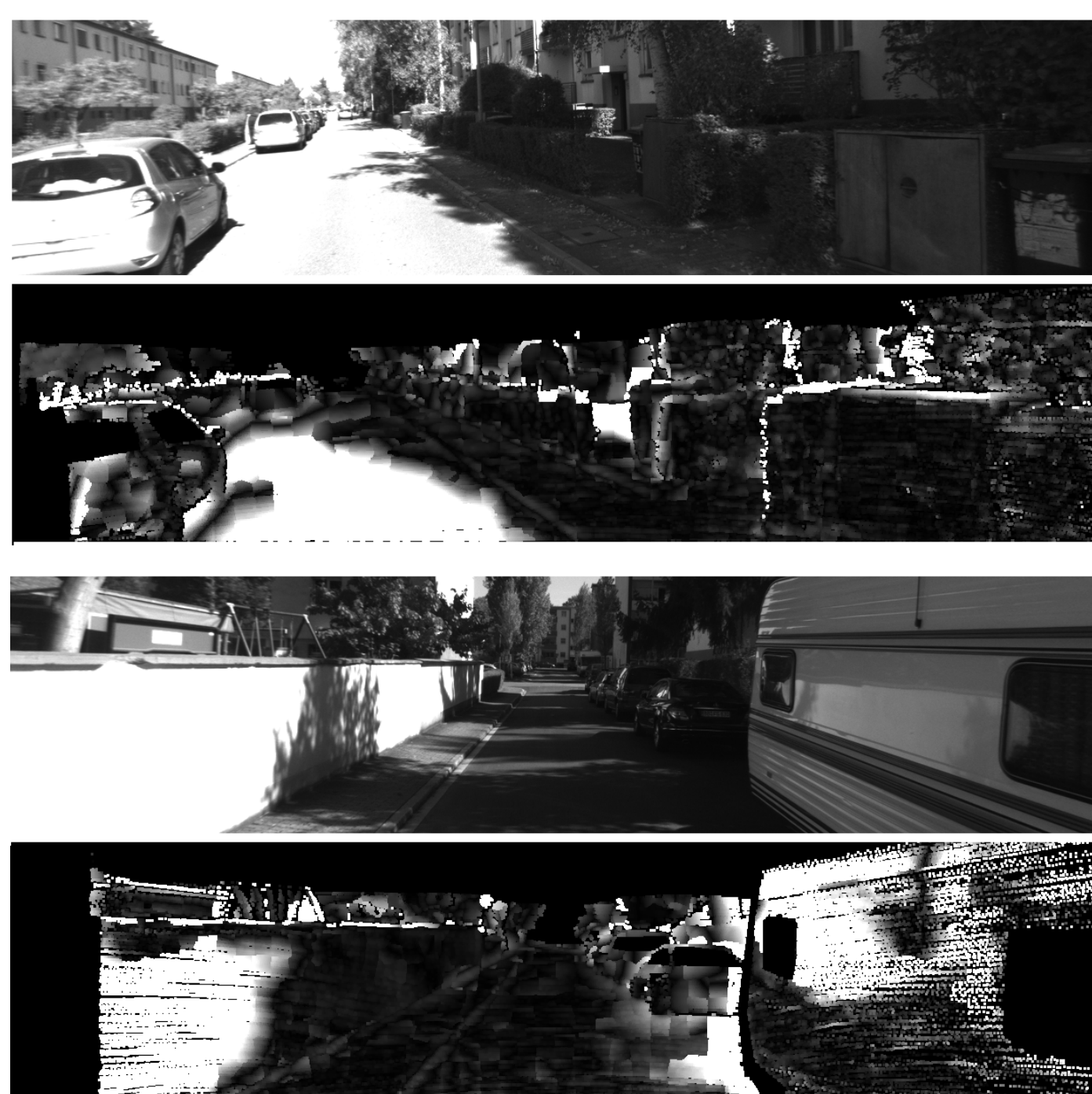
Stereo images from the KITTI benchmark and errors (white: >5px) made by the state-of-the-art methods.
