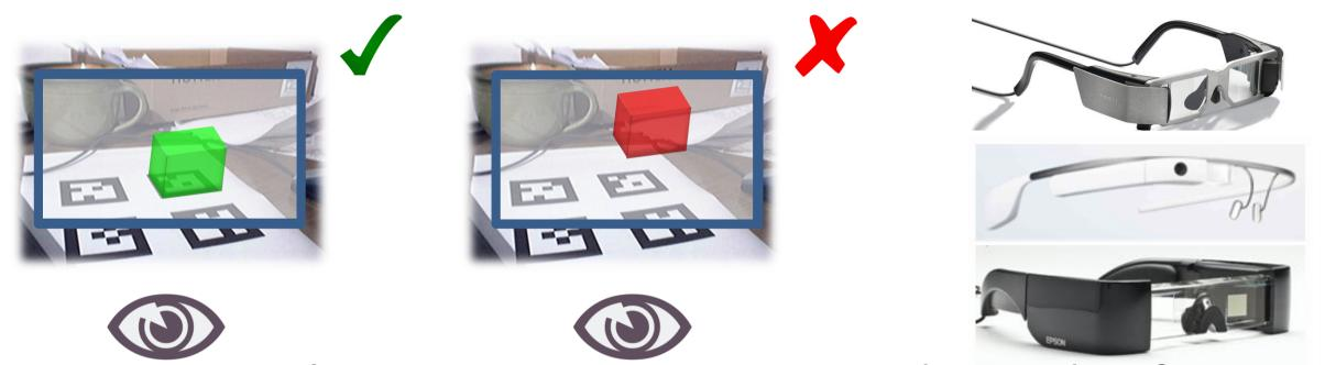
Maintaining the correct registration demands frequent (re)calibrations for the end-users whenever they move the HMD on their head (Touching, rubbing eyes etc.).
