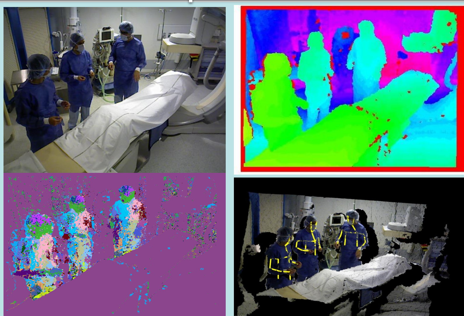
Input RGB and depth image, body part detector response and 3D skeleton overlaid on the reconstructed point cloud
