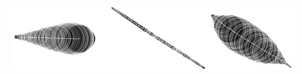
The width function is interpolated by Legendre polynomials. The vector of Legendre coefficients is referred to as the shape descriptor:
