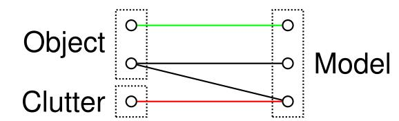
In our local matching technique, an initial estimate of the object is obtained by keypoint tracking. In a second step, implausible candidates for matching are removed and ambiguities are resolved.
