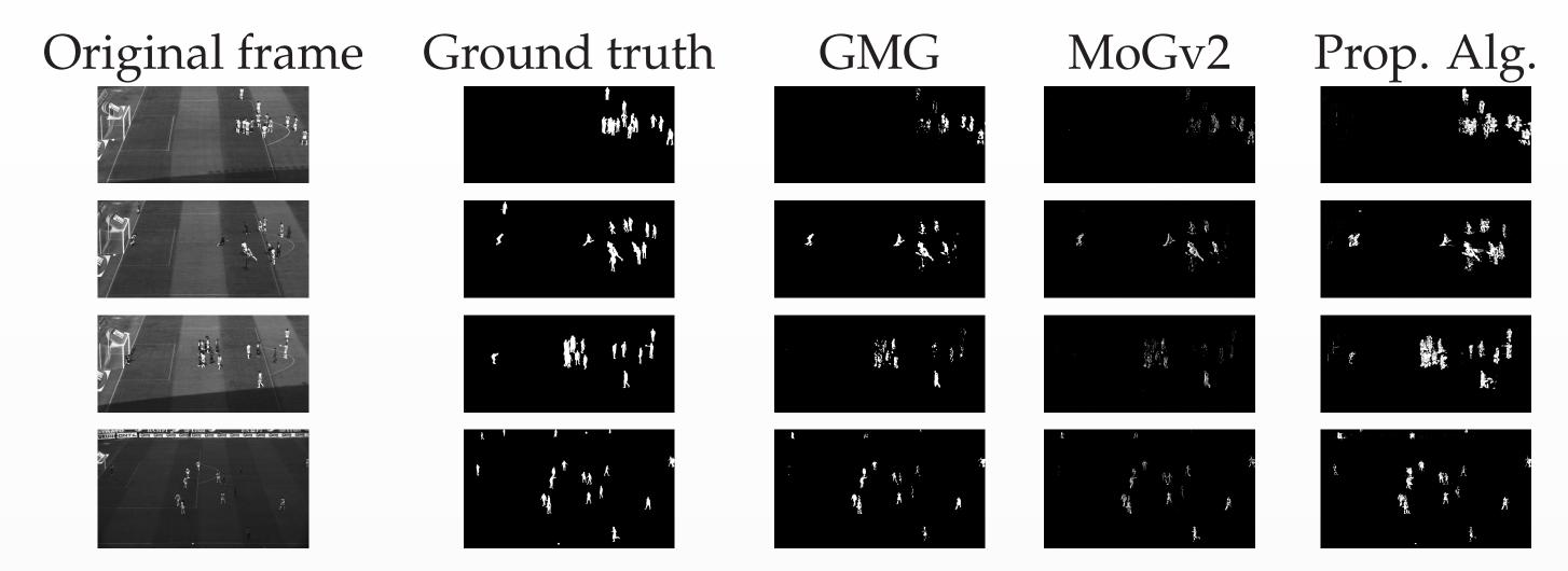
GMG [1] and MoGv2 [2] are implemented in the BGS Library [3]. The proposed algorithm is linear, fast and shows a good Recall. Its Precision is penalized, but can be improved with add-on modules.
