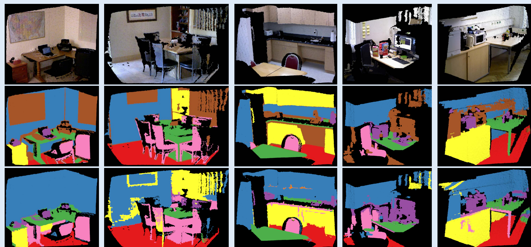
First row: input point clouds; second row: groundtruth; third row: results; first three columns: NYU v2; last two columns: our dataset.
